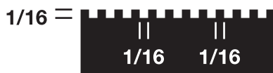
FELT-BACK ROTOVINYL SQ-NOTCH 1/16"D x 1/16"W x 1/16"A 140-160 sq. ft. (15-17 sq. yds.)/gal.
